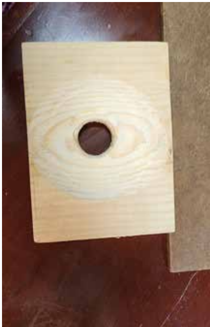
Removable 5 1/2" x 4" x 3/4 inch piece with sloping center around 1" hole lays over nestbox bottom. Care must be taken to align the holes.
